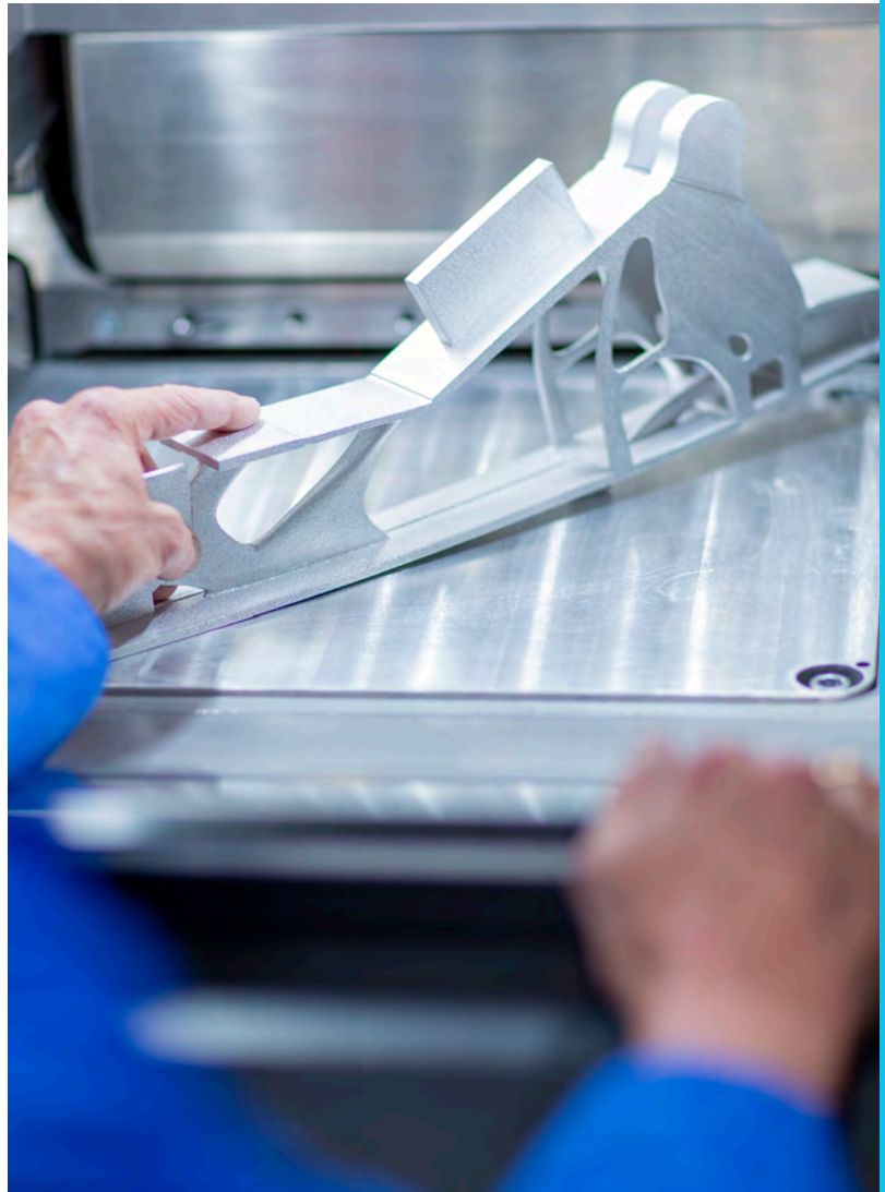
The lightweight component manufactured using laser sintering.
