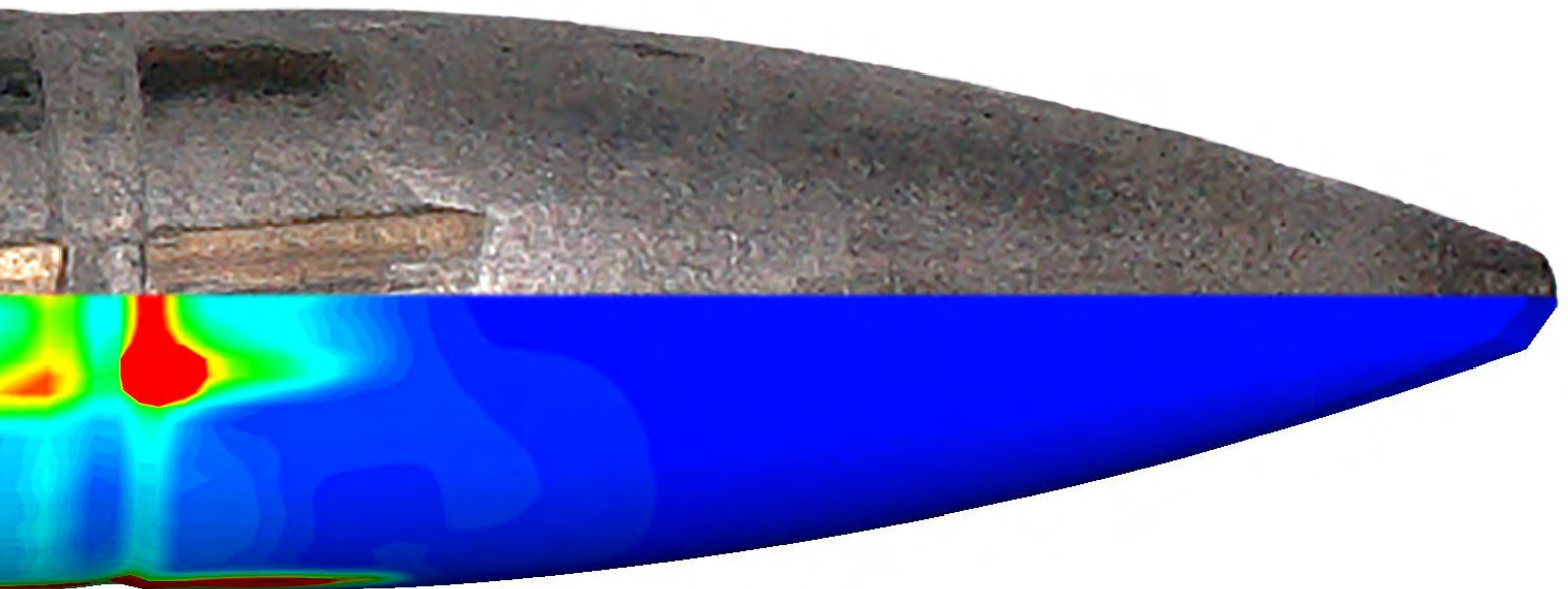
Deformation of a small-caliber projectile after firing in experiment and simulation.
