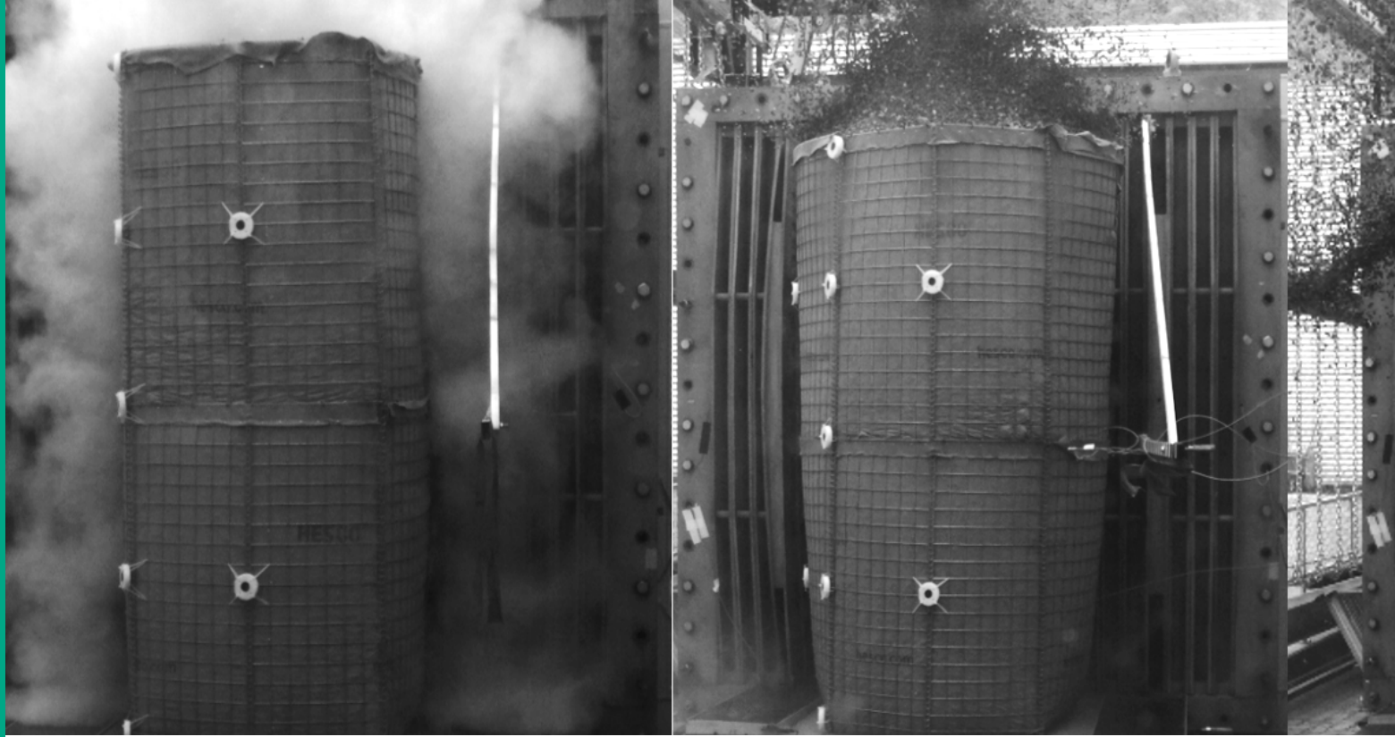
Investigation of the structural behavior of a soil-filled protective wall in a shock-tube test (detonation event in the far field).
